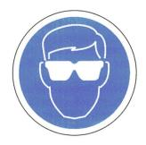
A sign prescribing a specific type of behaviour (i.e., Eye protection must be worn)
